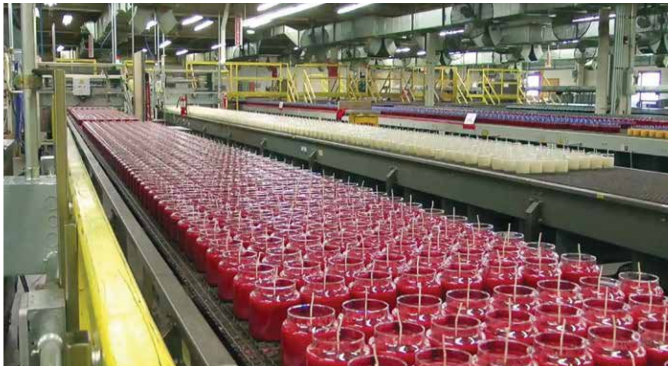
Jar candles, filled with coloured wax and wick, being mass produced in a candle factory. Exporters also add different fragrances to the candles, keeping with the demands of importers. The jars are made from non-inflammable materials.
